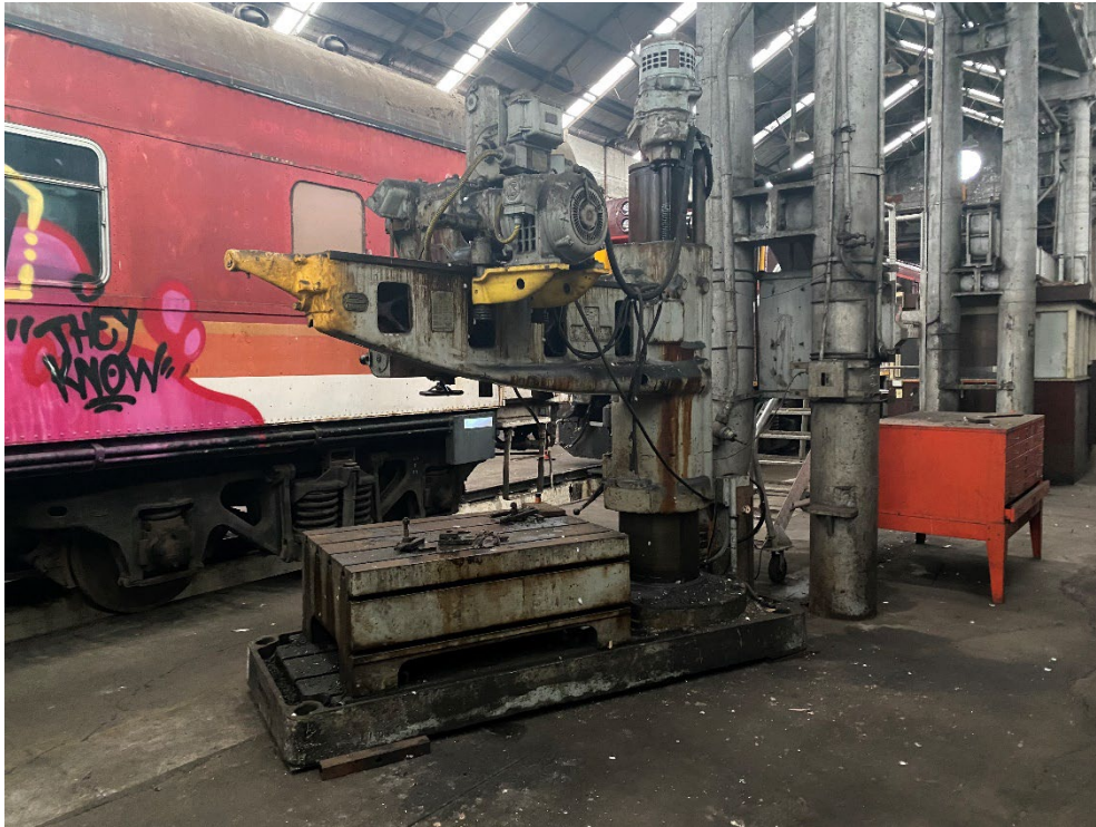
Figure 4.27: Drilling machine produced by William Asquith Ltd of Halifax, England, likely fabricated in the 1920s. The item is not listed as part of the ATP or Railcorp S170 Registers. Source: Curio Projects, 2022.
