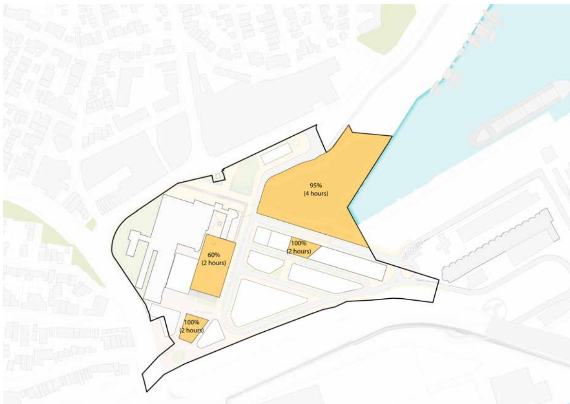
Figure 7.2.6: Proposed Solar Access to Public Open Space. The diagram shows solar access that is required in terms of proportions of the public open space that achieve a minimum of 2 hours direct sunlight between 9am and 3pm on 21st June (mid winter).
