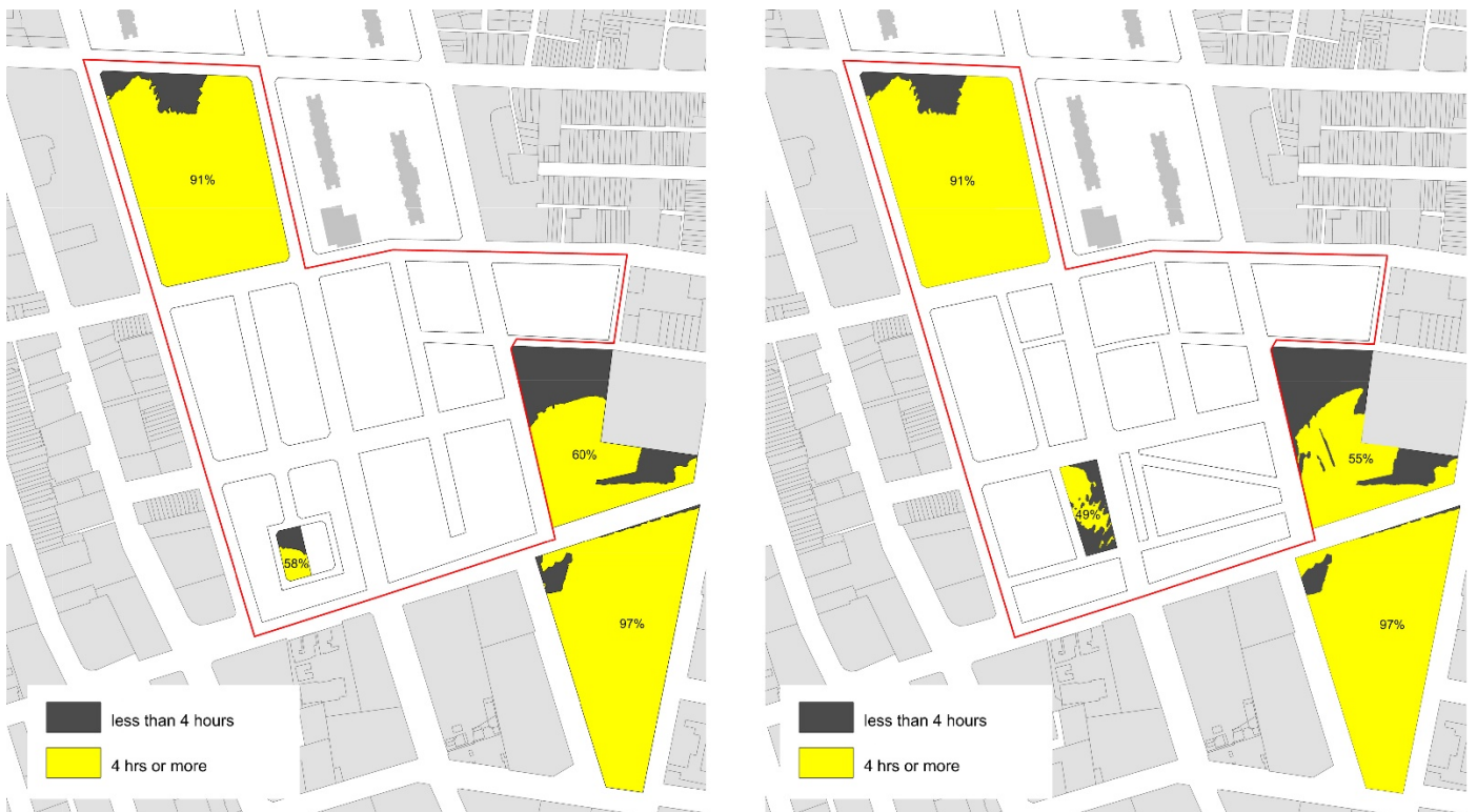
Area of parks receiving minimum 4 hours sunlight at the winter solstice (June 22)
