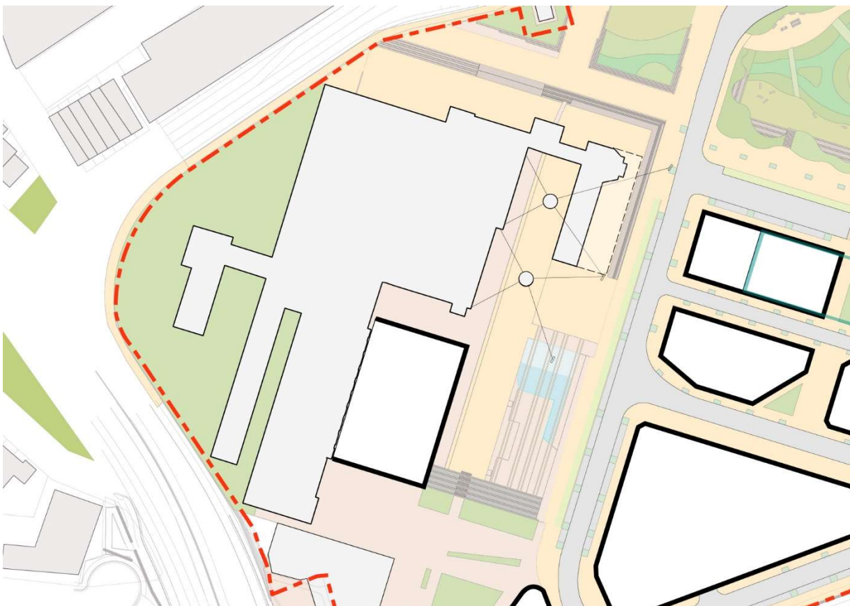
Figure 7 - White Bay Power Station New Boiler House - Primary Setback and Build To Line
