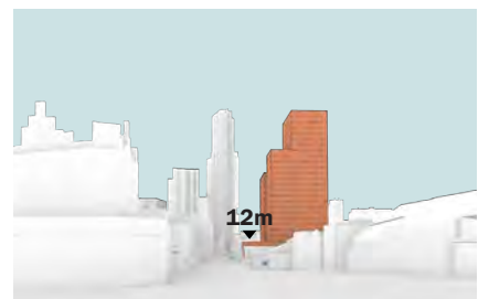
The tower near Prince Alfred Square is set back 12m from the street wall
