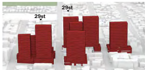
Potential resulting urban form along Church Street with base HOB 80m +12m DC bonus
