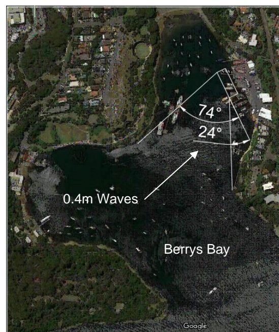
Figure 7.4: FDD in Berthing Pocket – 0.4m Wave Direction
