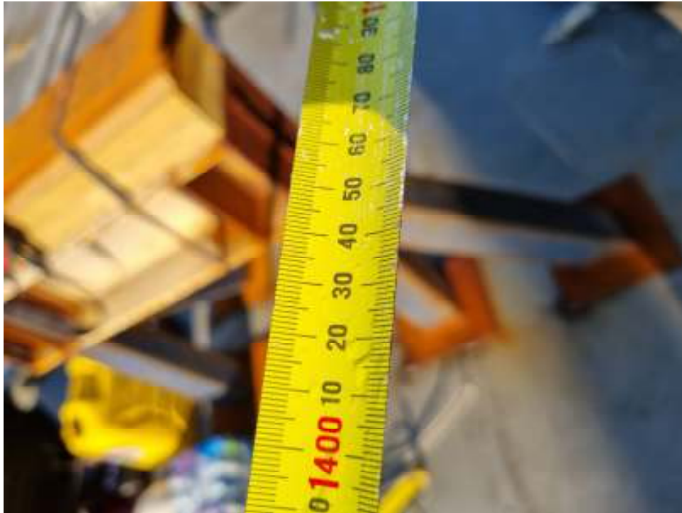
Figure B21: Transfer Tank 7 Sounding, Initial condition (1442mm)
