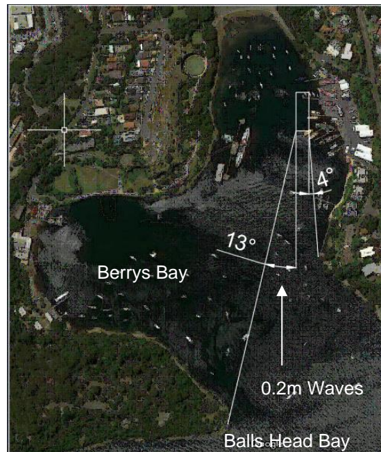
Figure 7.3: FDD in Lifting Pocket – 0.2m Wave Direction
