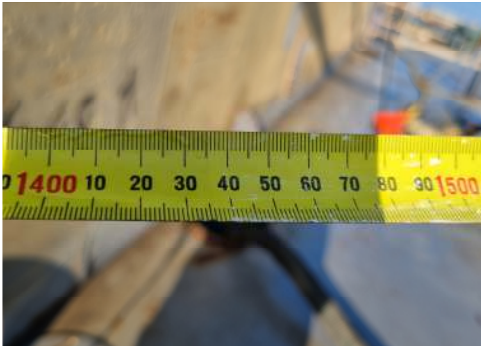
Figure B23: Transfer Tank 9 Sounding, Initial condition (1439mm)
