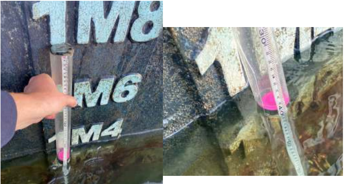
Figure B9 Draft measurement Port Fwd (1M8 – 392)
