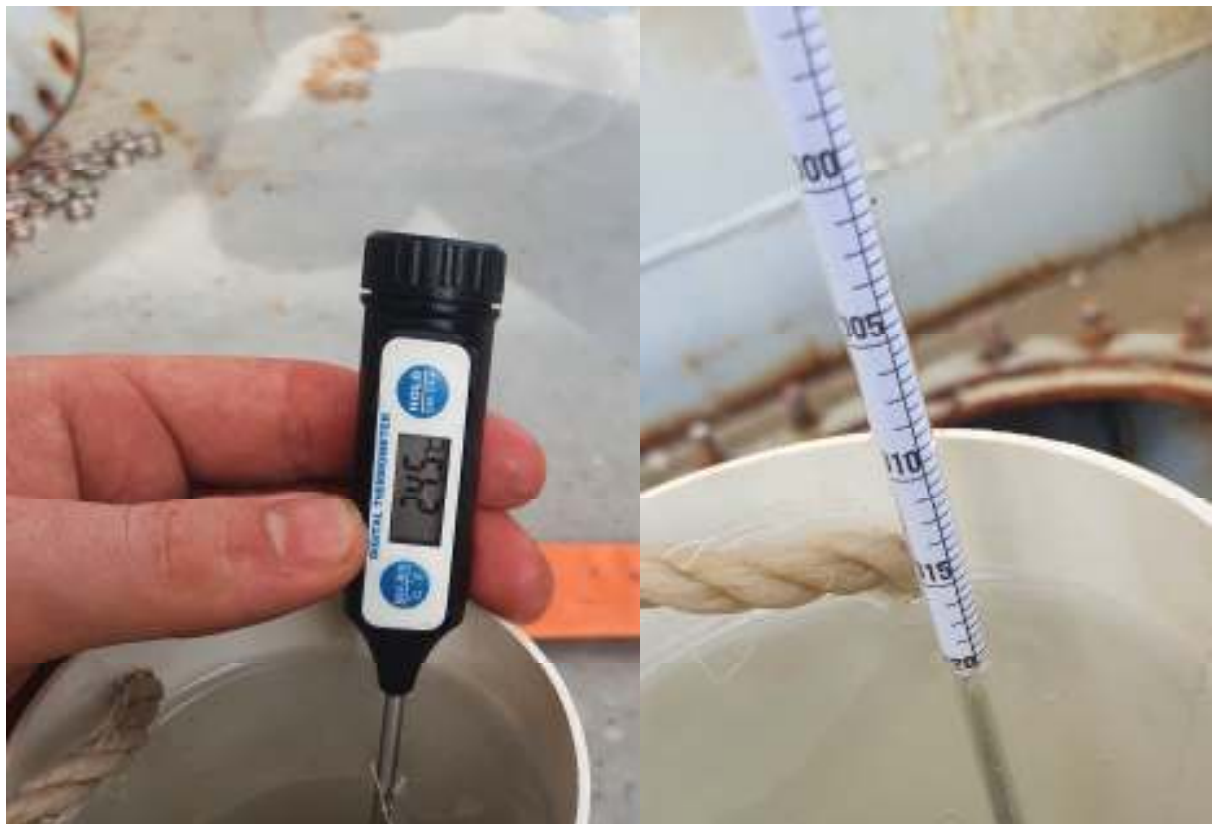
Figure B14: Typical Tank Density and Temperature Reading
