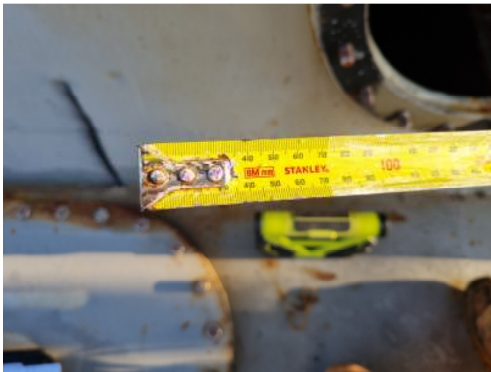
Figure B24: Tank 10 Sounding (72mm)
