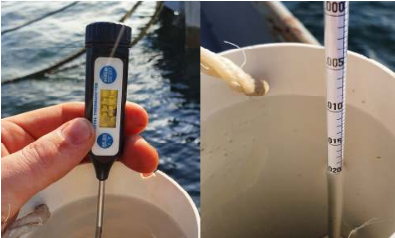
Figure B13: Typical Ocean Density & Temperature Reading
