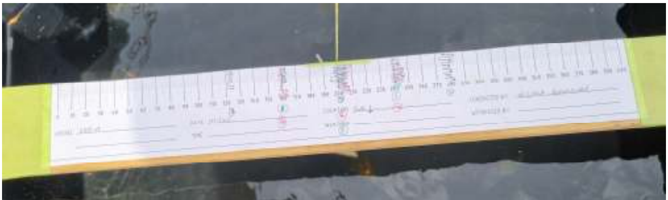
Figure B6: Fwd Pendulum measurement strip
