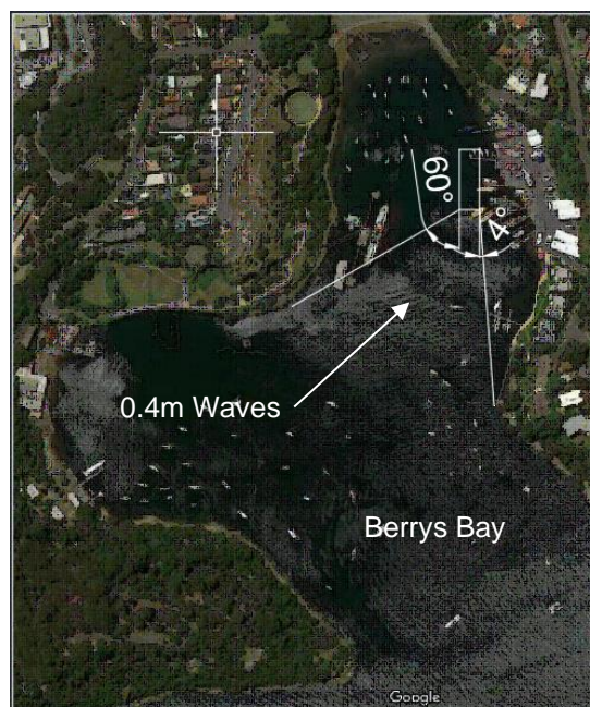
Figure 7.2: FDD in Lifting pocket – 0.4m Wave Direction
