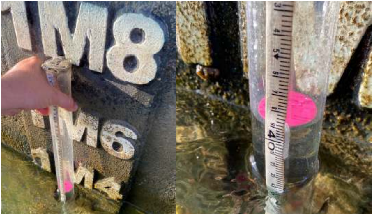
Figure B11: Draft measurement Stbd Mid (1M8 – 391)
