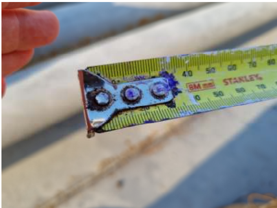
Figure B22: Tank 8 Sounding (34mm)
