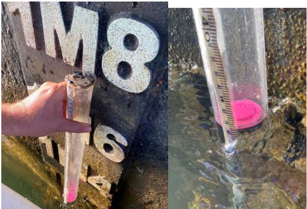
Figure B10: Draft measurement Stbd Fwd (1M8 – 472)
