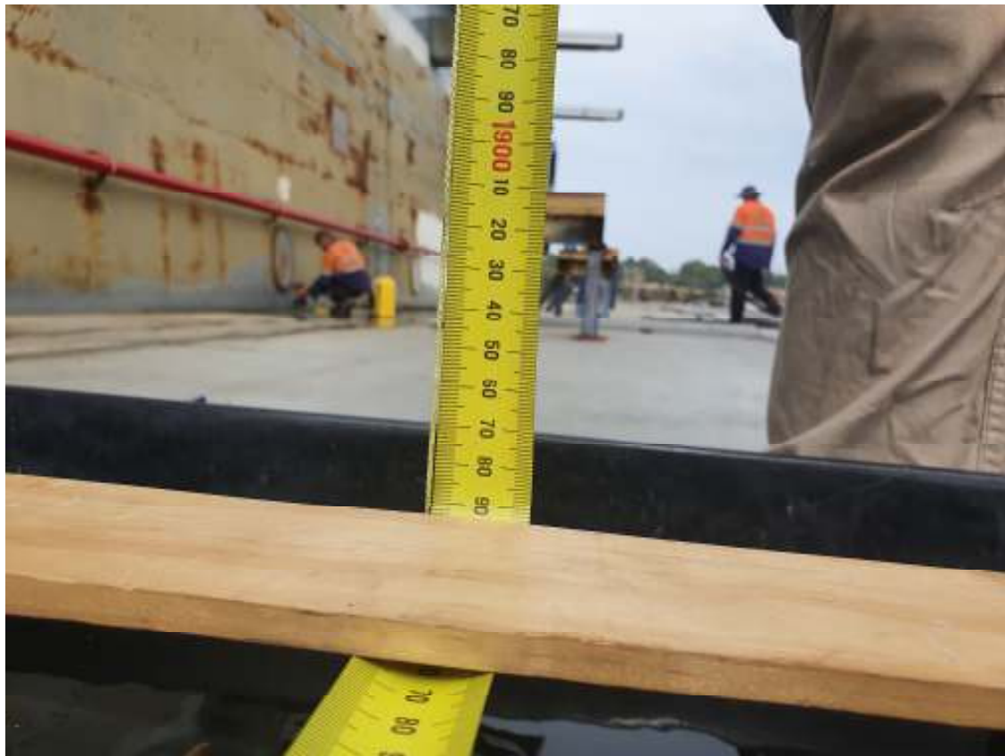
Figure B5: Fwd Pendulum length measurement
