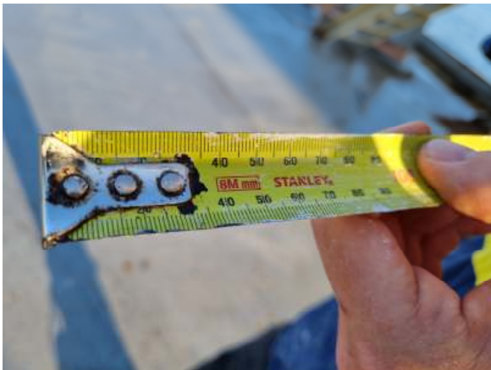
Figure B16: Tank 2 Sounding (35mm)
