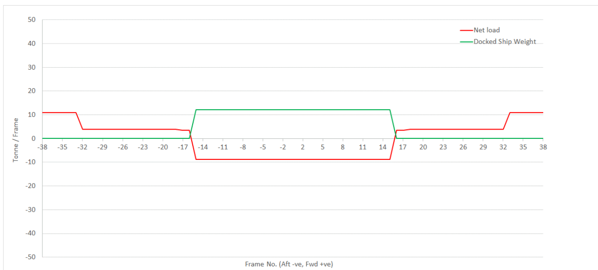
Figure 4.8.1.7 Load Distribution – Paluma Class Surveying Ship
