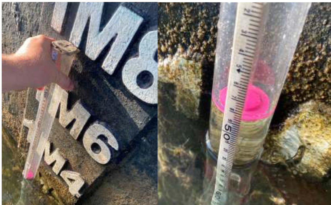
Figure B12: Draft measurement Stbd Aft (1M8 – 485)
