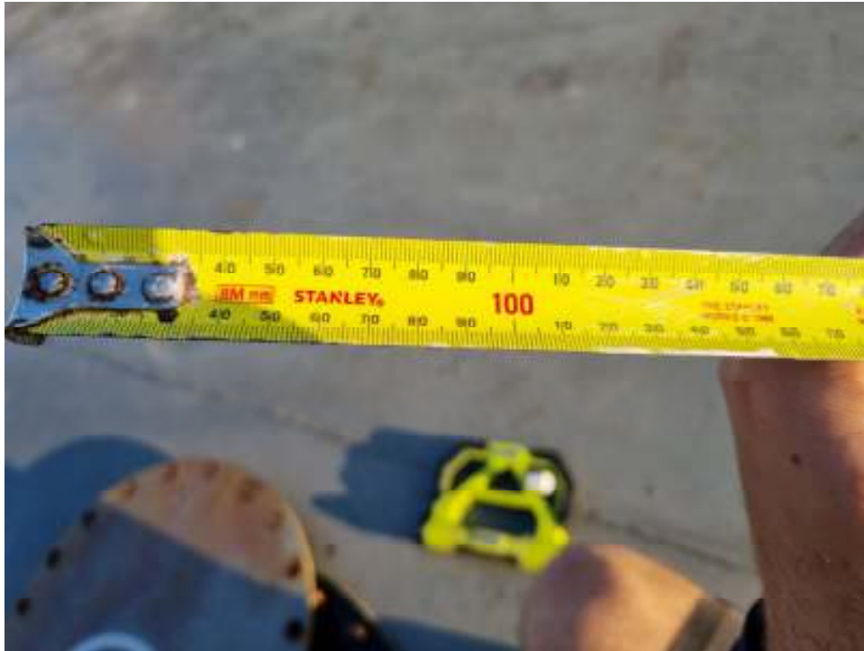
Figure B19: Tank 5 Sounding (88mm)
