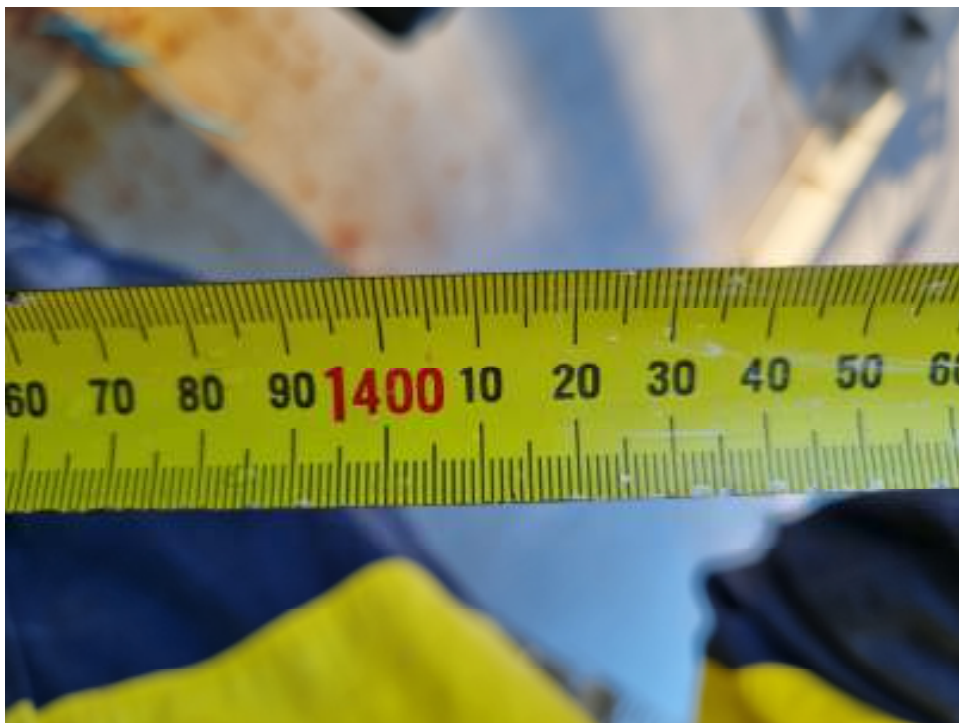
Figure B18: Transfer Tank 4 Sounding, Initial condition (1417mm)
