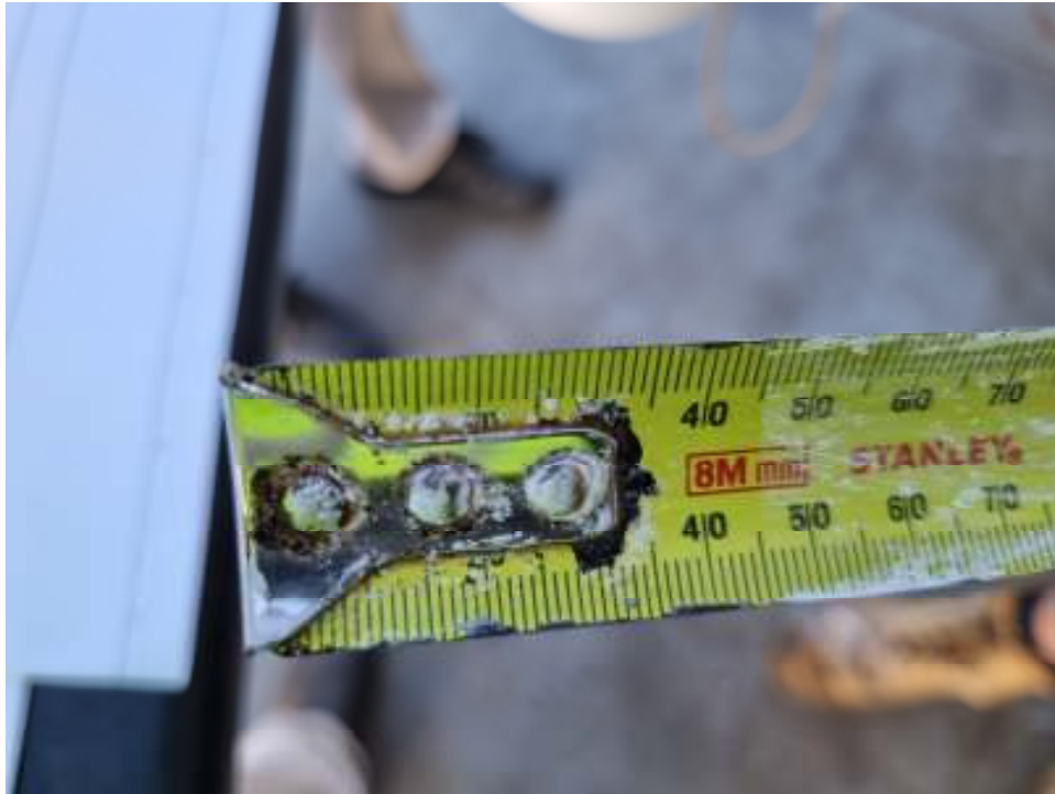
Figure B15: Tank 1 Sounding (44mm)
