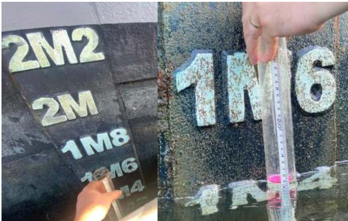
Figure B8: Draft measurement Port Mid (1M8 – 290)
