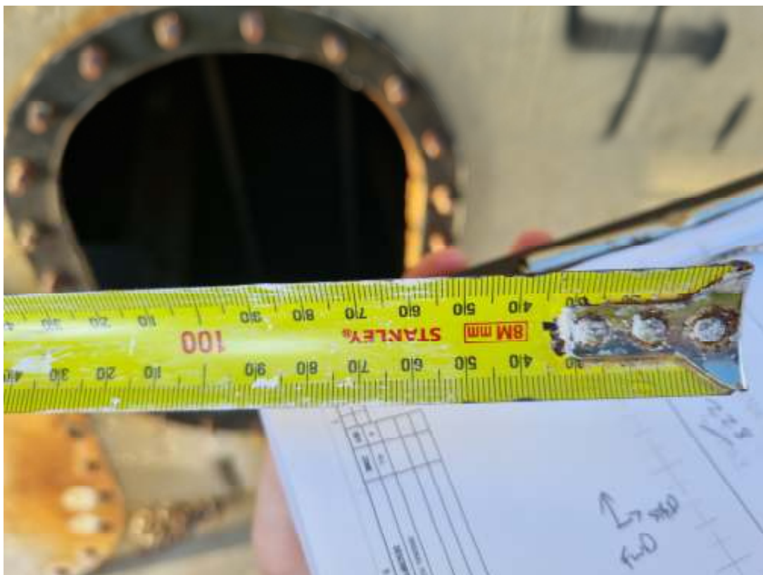
Figure B26: Tank 12 Sounding (52mm)
