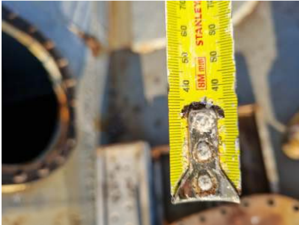
Figure B17: Tank 3 Sounding (39mm)
