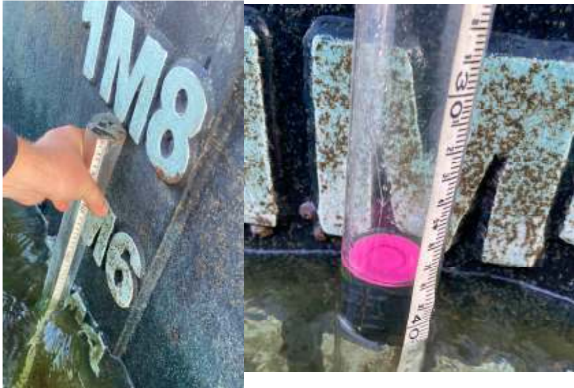
Figure B7: Draft measurement Port Aft (1M8 – 375)
