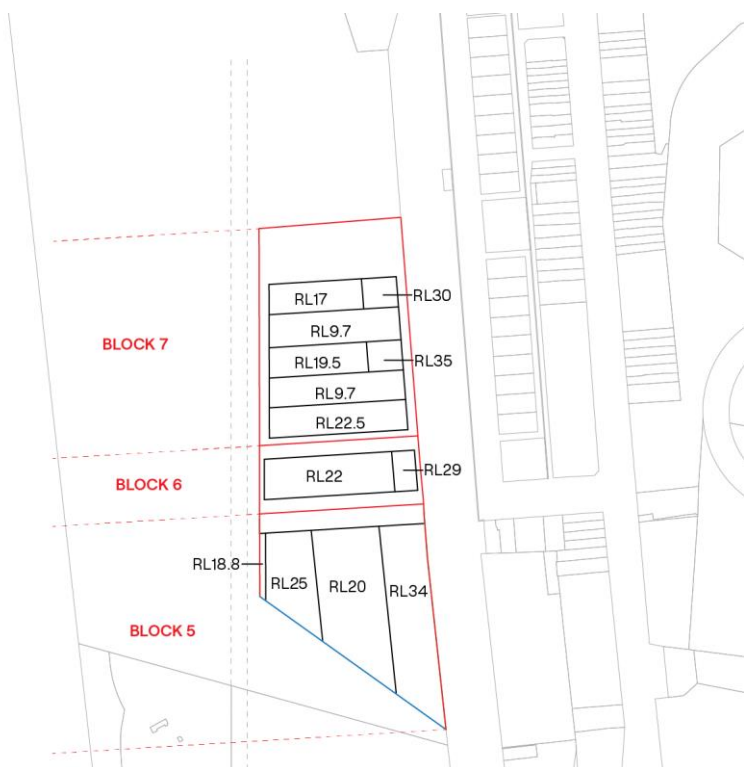
Figure 10: Indicative Built Form under Modification 8; southern boundary of Block 5 is chamfered. (Source: Gyde Consulting).
