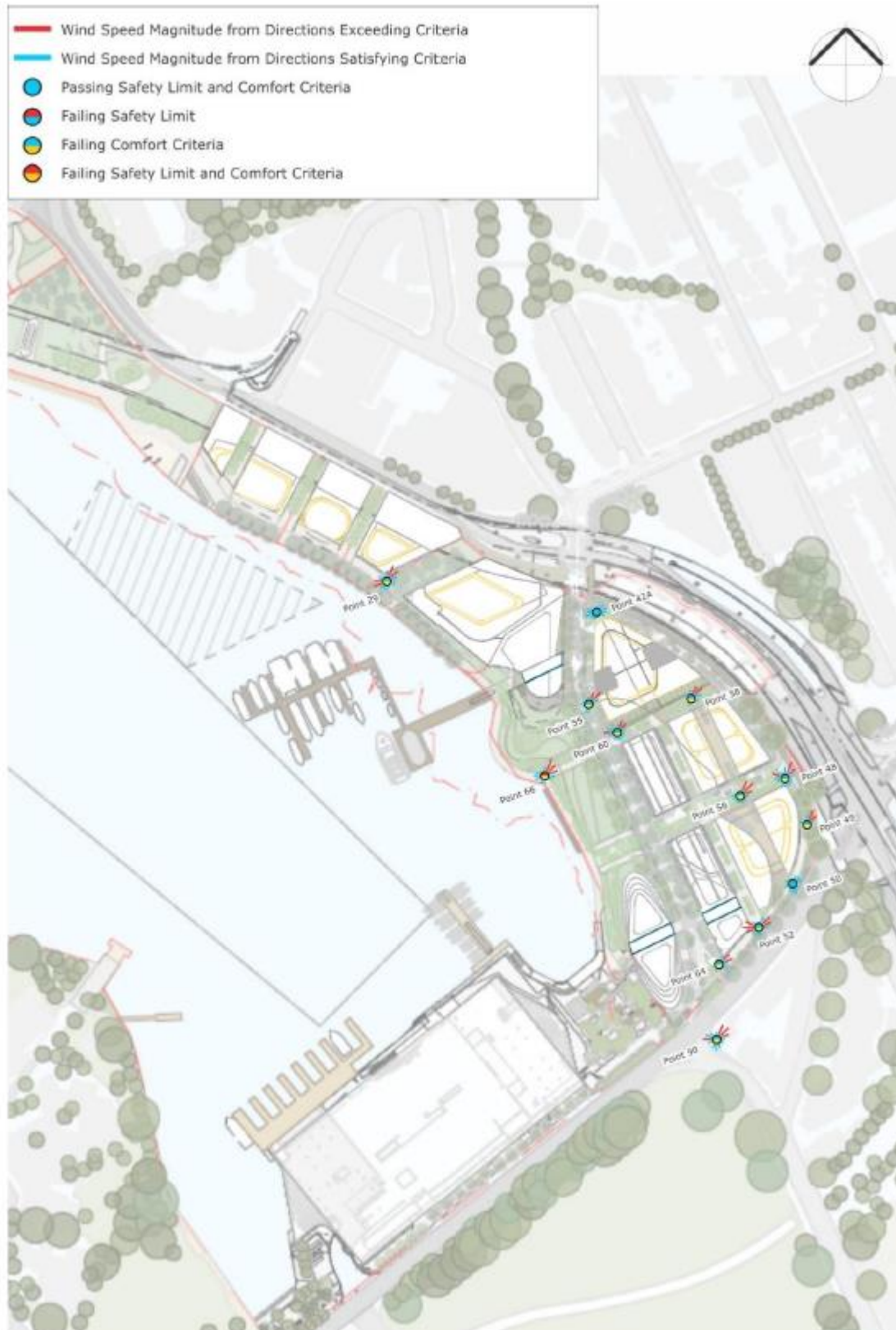
Figure 69: Wind tunnel results with treatments added (Source: Windtech)
