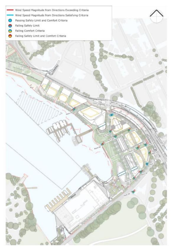
**Figure 69:** Wind tunnel results with treatments added (Source: Windtech)
