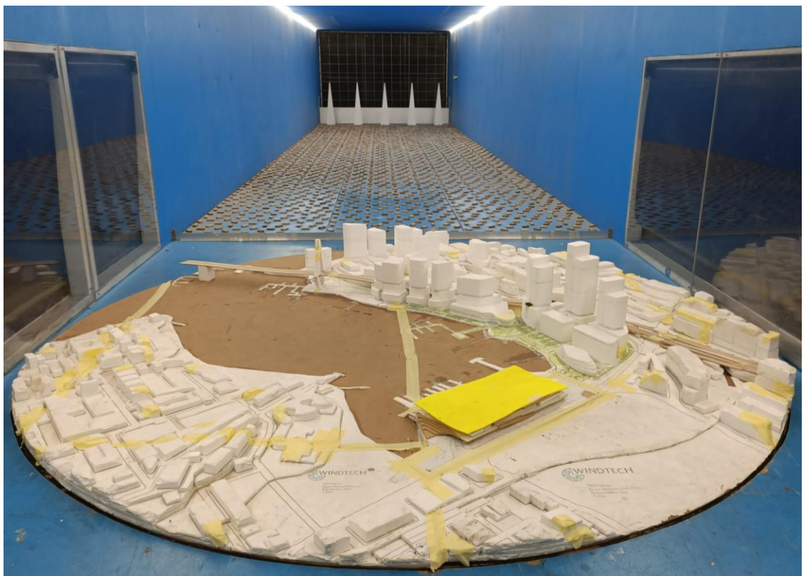
Figure 1a: Photograph of the Wind Tunnel Model (proposed scenario, view from the south)
