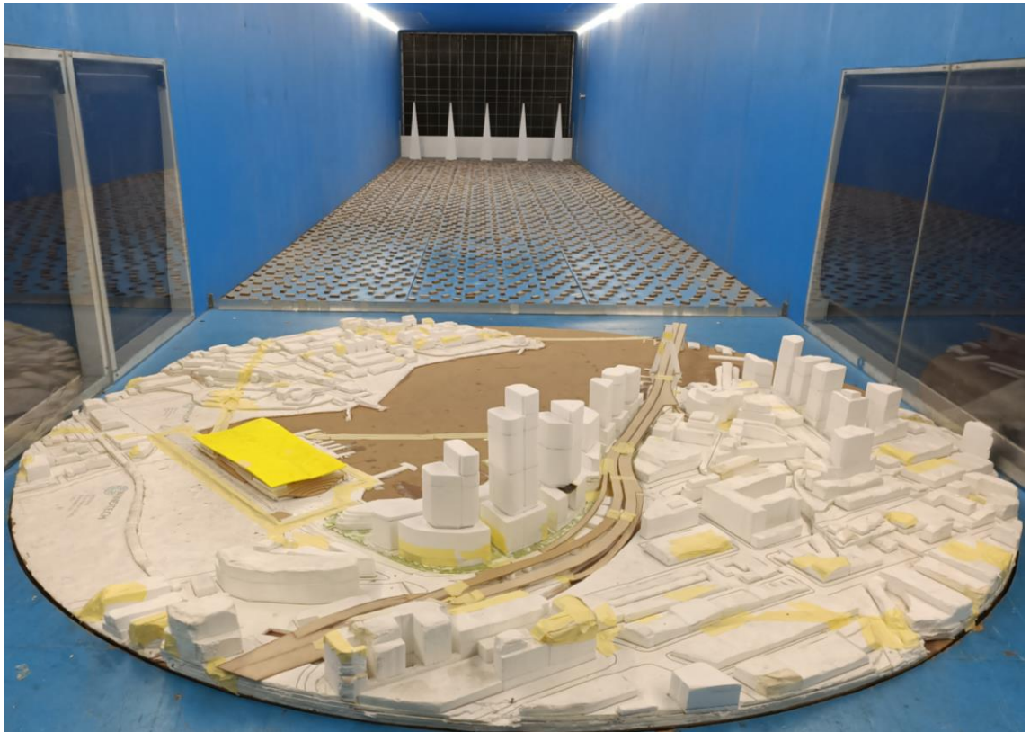
Figure 1d: Close up photograph of the Wind Tunnel Model (proposed scenario, view from the east)
