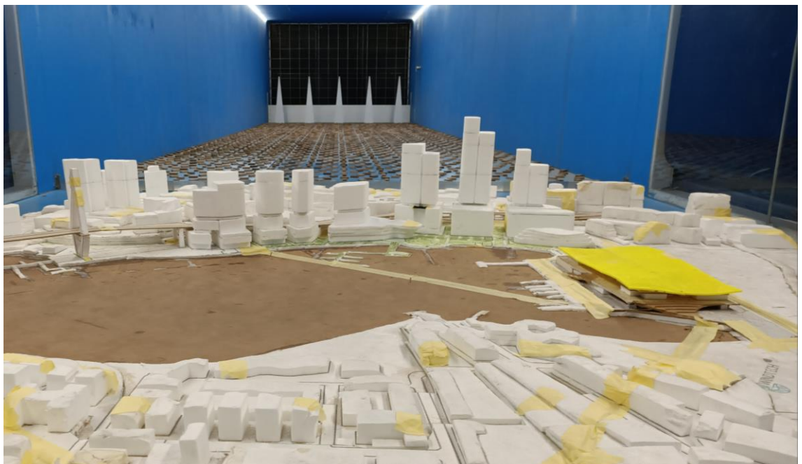
Figure 1e: Close up photograph of the Wind Tunnel Model (proposed scenario, view from the south-west)
