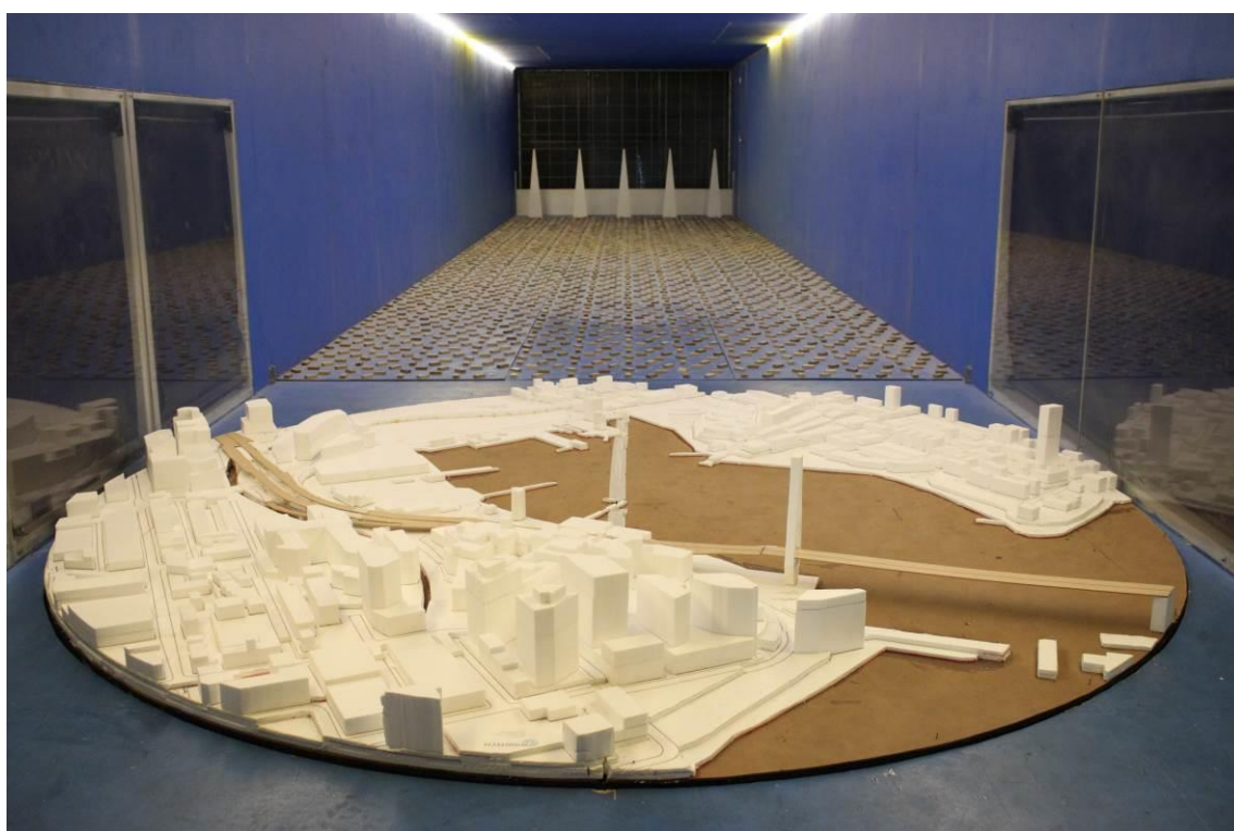
Figure 2a: Photograph of the Wind Tunnel Model – (View from the north)
