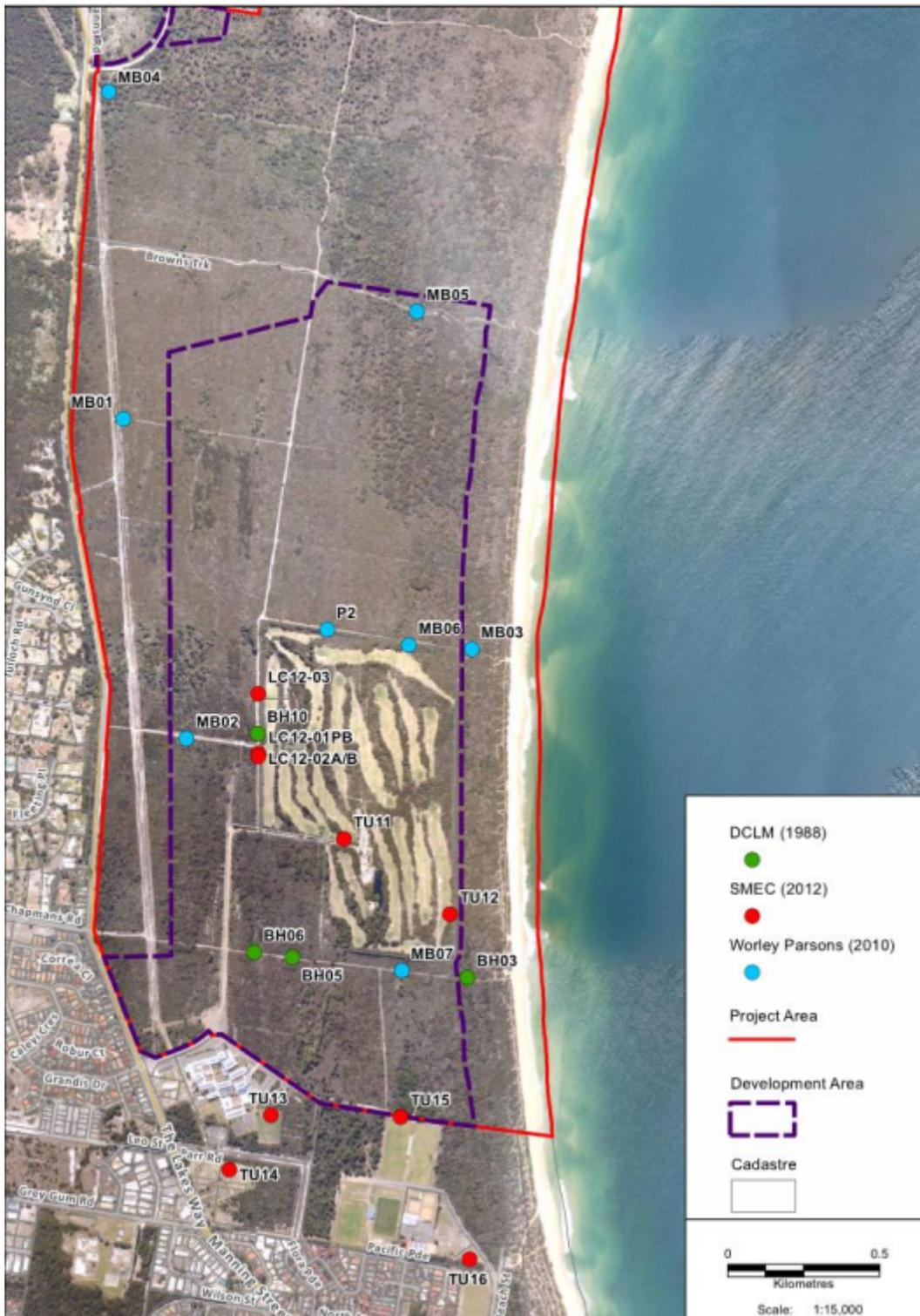
**Plate-5 – Location of Groundwater Monitoring Bores**
