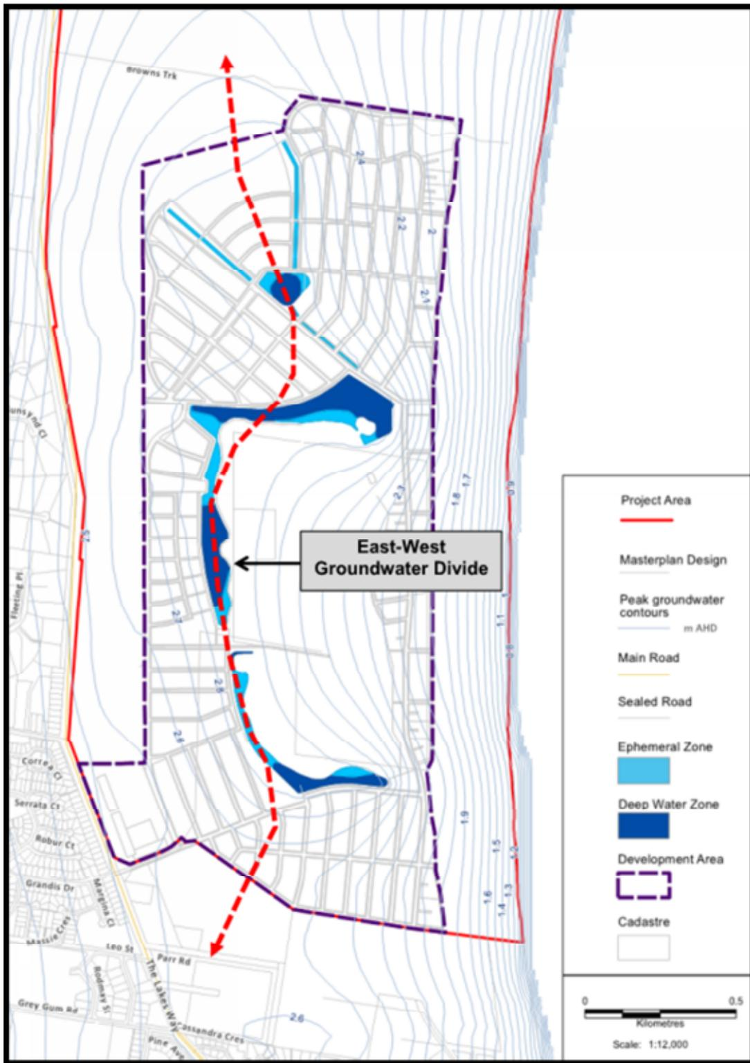
**Plate-3 – Developed conditions detailed groundwater model results: Typical 90<sup>th</sup> Percentile (wet weather) groundwater conditions (SMEC, 2014)**
