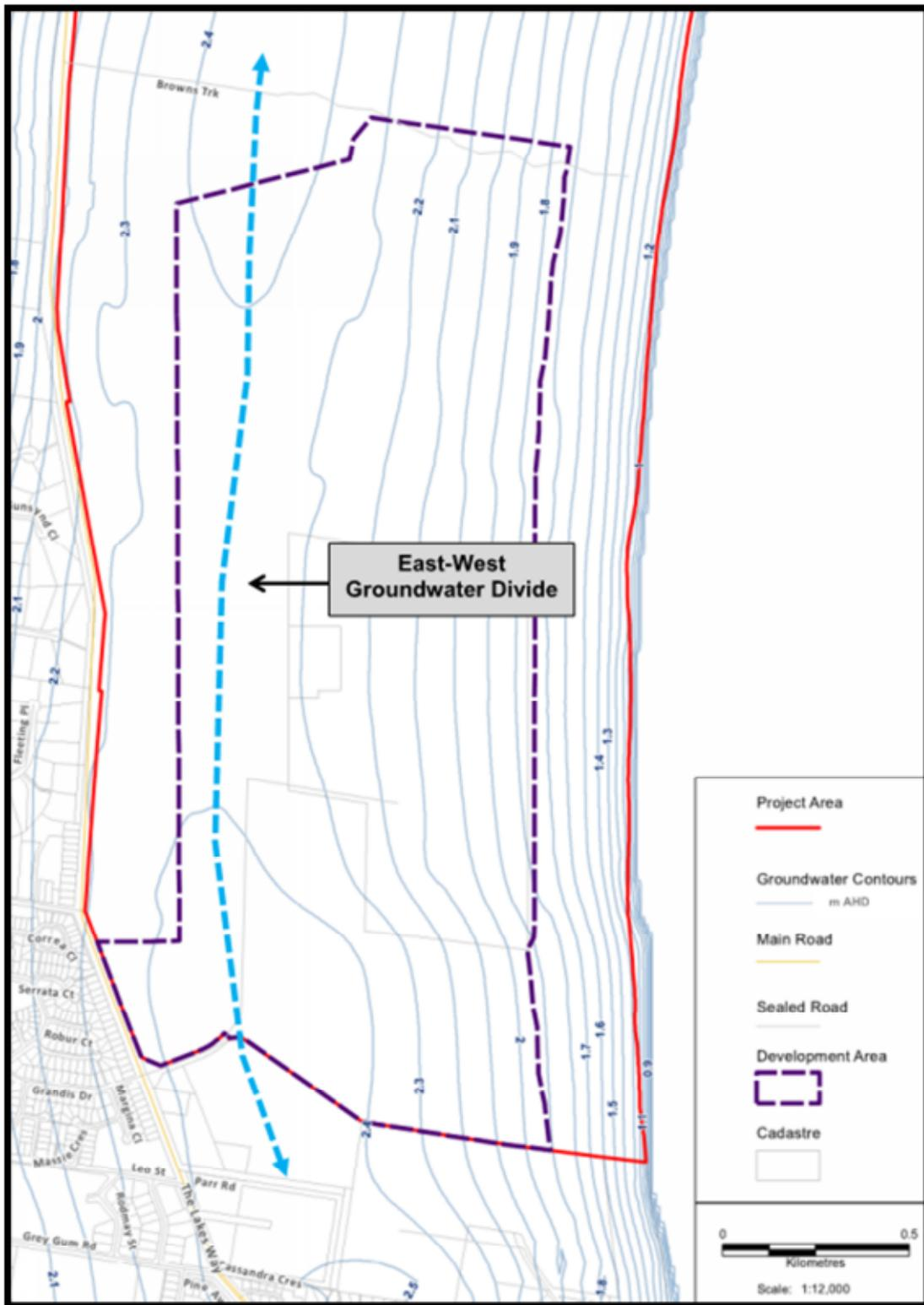
**Plate-2 – Indicative groundwater profile on 24 July 2011 following a groundwater recharge event (SMEC, 2014)**
