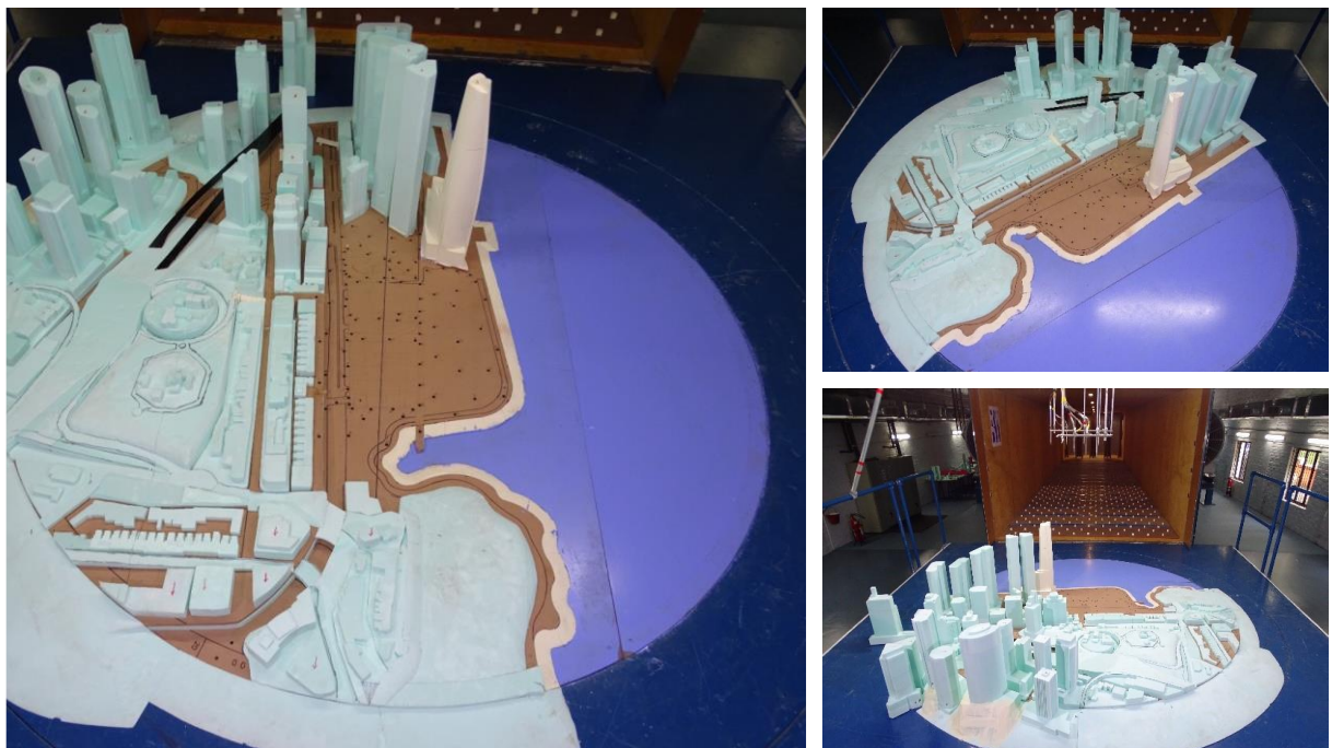
Image 2A: Wind Tunnel Study Model – Existing Configuration
