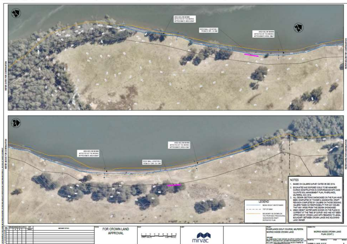
FOR CROWN LAND APPROVAL SPRINT 41-12 FOR CONTINUATION LEGEND PROPOSED ROAD LAYOUT BOUNDARY OF CROWN LAND BOUNDARY OF MURRUMBIDGEE RIVER NOTES 1. BASED ON CALSURE SURVEY DATED 19 DEC 2016 2. EXISTING AND EXPOSED SOIL TO BE REMOVED DURING CONSTRUCTION IN CONFORMANCE WITH SOIL EROSION MANAGEMENT PLAN, MURRUMBIDGEE, MURRUMBIDGEE, NSW 2515 3. ALL DESIGN SECTIONS SHOWN ON THE PLAN HAVE BEEN COMPLETED BY TONKIN LANDSCAPE ARCHITECTS, SMITH PERKINS COMPLETED BY CALSURE ON THOSE DESIGN SECTIONS COMPLETED BY CALSURE FOR ANY DESIGN THAT MAY ARISE FROM THE DESIGN SHOWN ON THE PLAN IS CURRENT AT THE TIME OF SURVEY AND HAS NOT BEEN APPROVED BY CROWN LAND WITH REGARD TO LEGAL BOUNDARY BETWEEN CROWN LAND AND ADJOINING LAND OWNER SCALE 0 10 20 30 40 50 60 70 80 90 100 METRES PROPOSED ROAD LAYOUT BOUNDARY OF CROWN LAND BOUNDARY OF MURRUMBIDGEE RIVER SPRINT 41-12 FOR CONTINUATION
