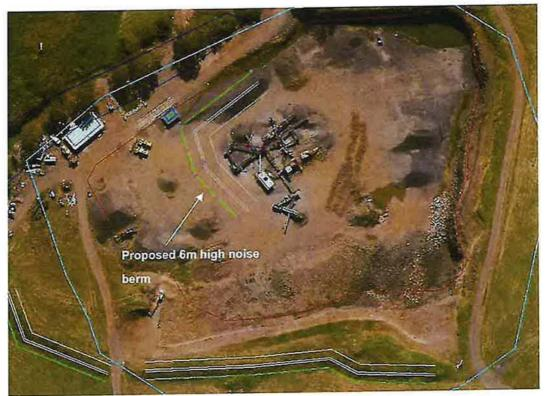
Figure 11 | Proposed noise berm in quarry pit
