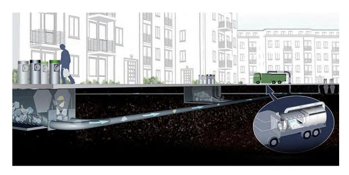
Local Collection System Underground Tanks and Mobile Vacuum Truck
