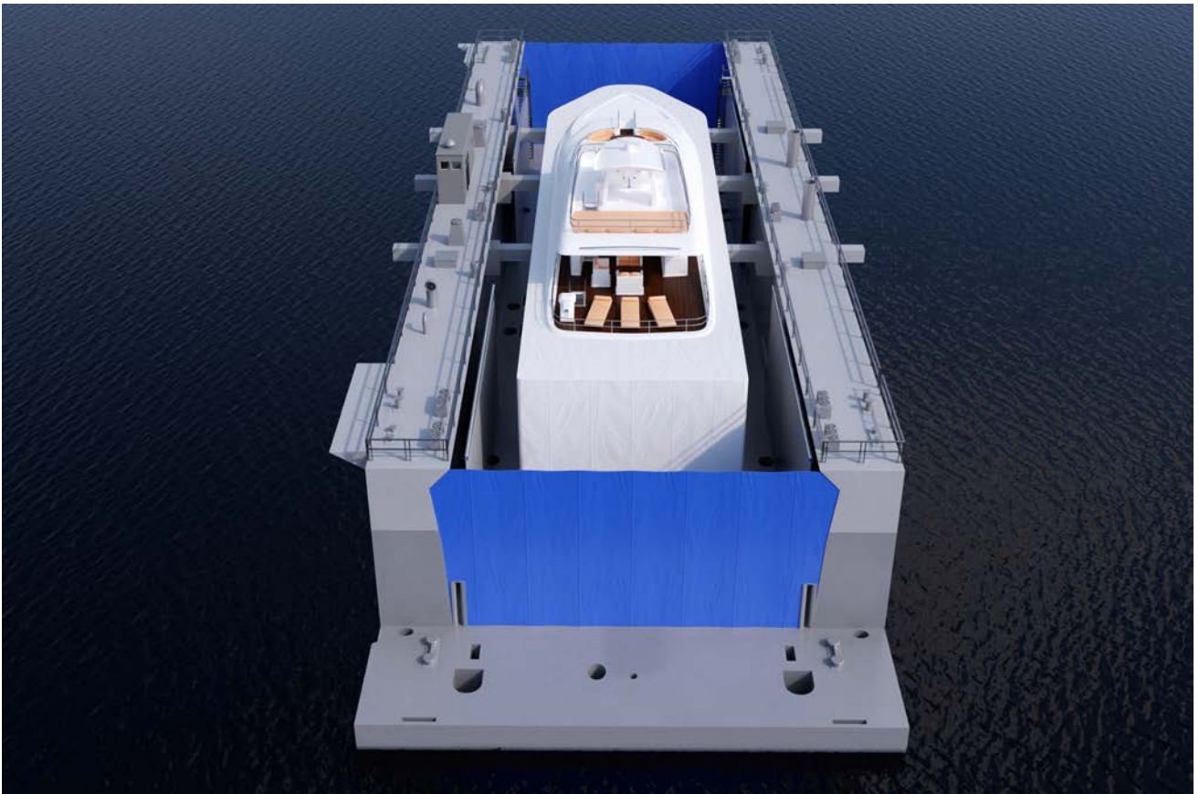
Front aerial view showing acoustic curtains and partial encapsulation.
