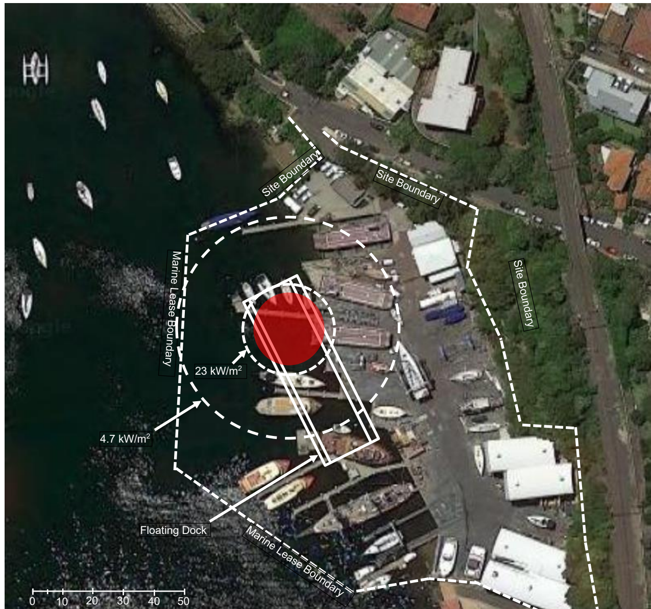
Figure 5.10: Heat Radiation Impacts – Vessel (Ship/Boat) Fire in the Fibre-Glass Hull
