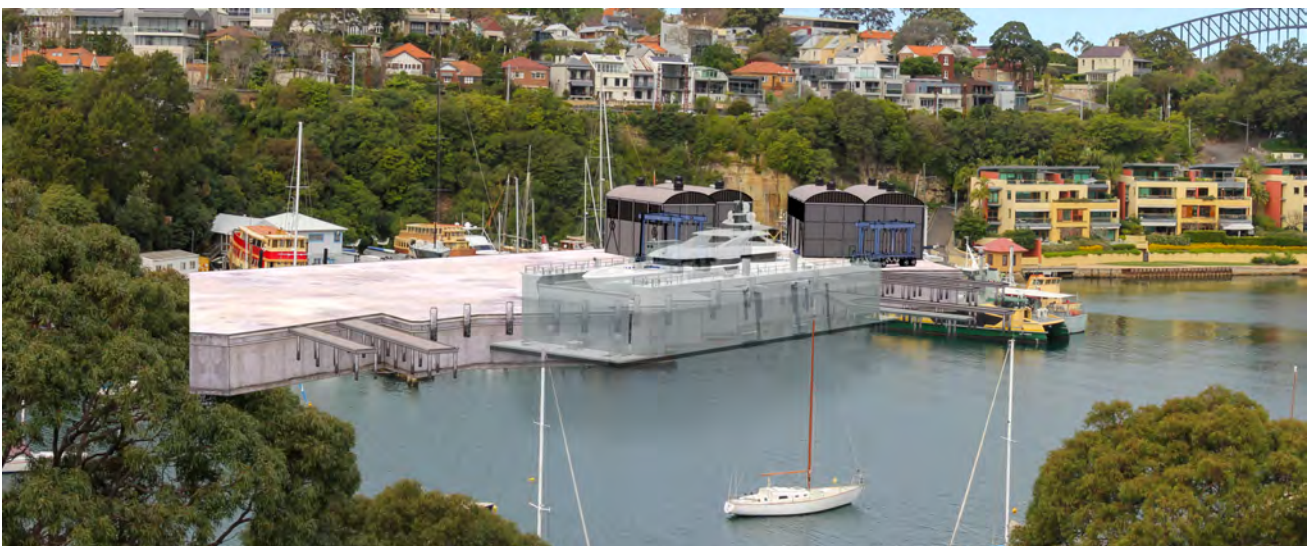
Original photo with 3D CAD modelling aligned to 3d survey
