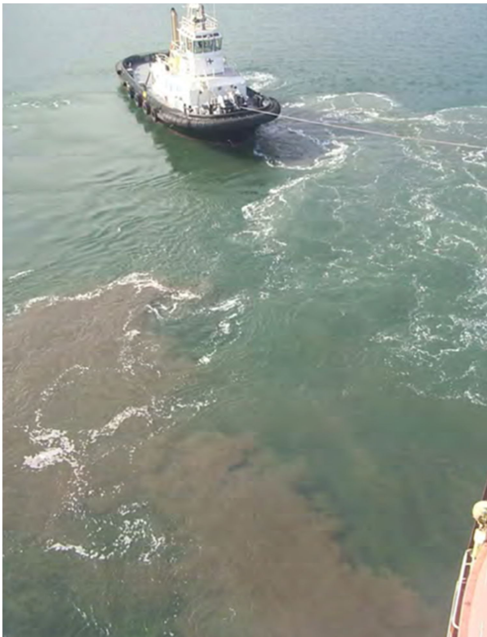
Figure 2 Cruise Ship Propeller plume at Circular Quay (from Knott and Johnston 2010).
