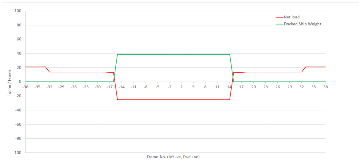
Figure 4.8.1.3 Load Distribution – Harbour tug
