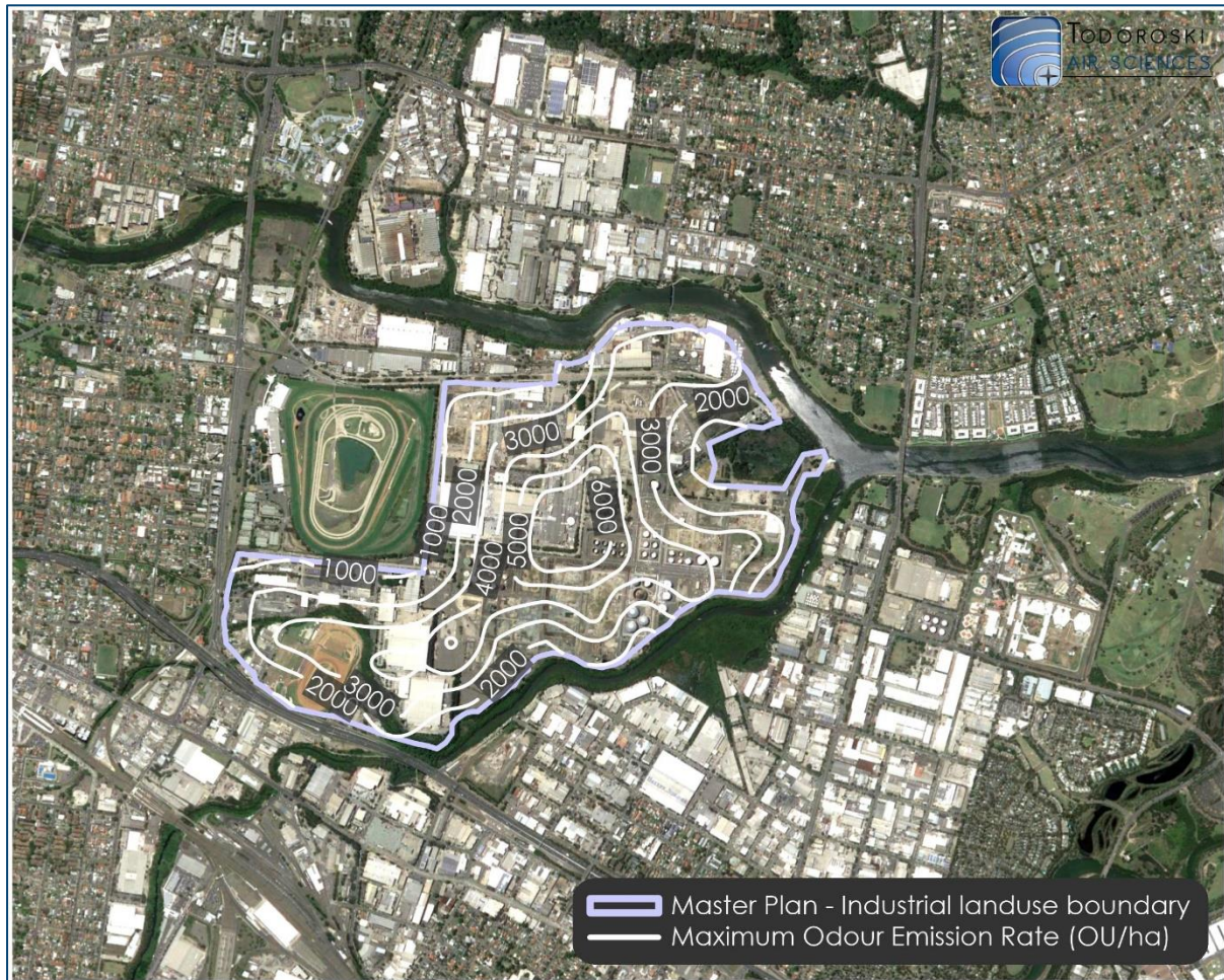
Figure 5-1: Source odour emissions rate per Ha (left) from the industrial area
