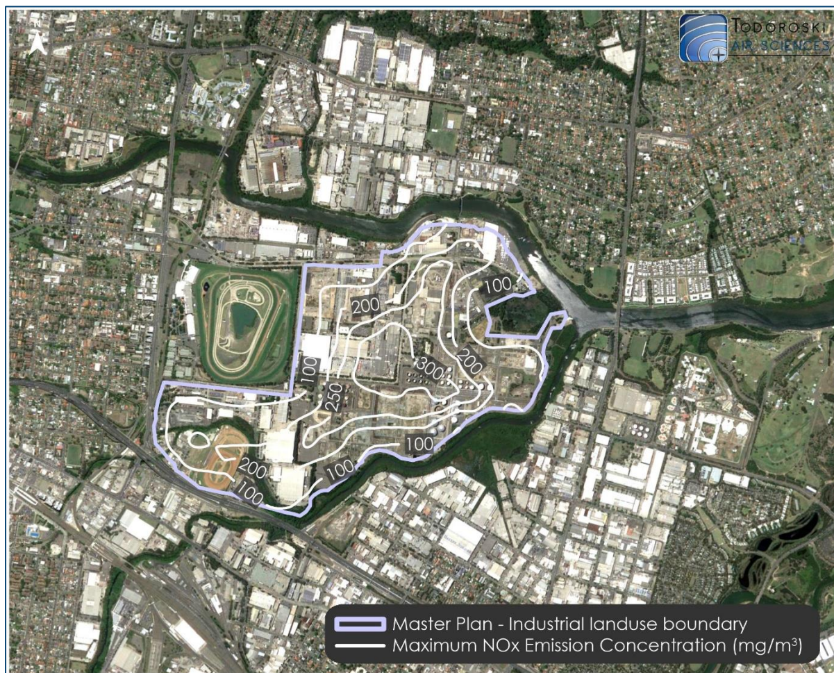
Figure 5-3: Air emission concentration per stack from the industrial area
