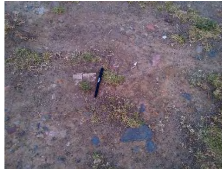
130 O'Connell St, Suspected ACM exposed on ground surface, car park and stockpiled waste in south-east of the site (POI BA)
