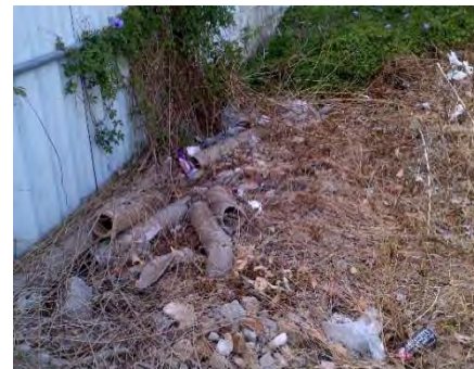
130 O'Connell St, Suspected ACM exposed on ground surface, car park and stockpiled waste in south-east of the site (POI BA)
