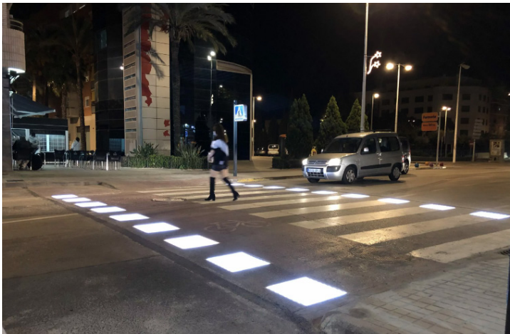
Figure 2.4 Smart road marking for pedestrian crossing (Source: STEPVIAL)
