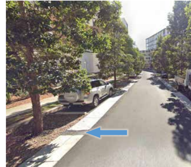
Passive street tree irrigation: Healthy and vigorous street tree planting on nearby Maryland Street benefiting from pits collecting stormwater runoff and supplying each tree. Other streets nearby where these techniques have not been used have trees that are much smaller.
